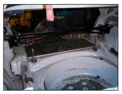
**Step 7:** Prior to installing the lower floor/subspace frame support you must thread the 9" long steel rods completely flush with the subfloor.
