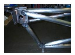
Step 11: Seat all bolts until tight. Take care to avoid over-tightening which can result in gauling or stripping of the bolts. Mason Engineering recommends a test drive of your vehicle followed by a recheck of all connections ensuring they are correct.
