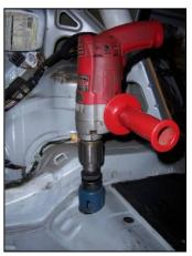
**Step 4 (option 1):** The sub frame mount holes are only partially threaded; there is approximately <sup>1</sup>/<sub>4</sub>" of non-tapped hole at the trunk end of the hole. To install your Mason Engineering lower floor/subspace frame support it is necessary to thread the remainder of
